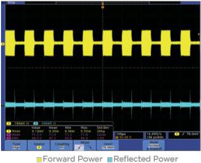
Navigator® II matching network: advanced algorithms allow for active tuning during a pulse · Increased stability · Improved reliability with less cycling · Less reflected power
